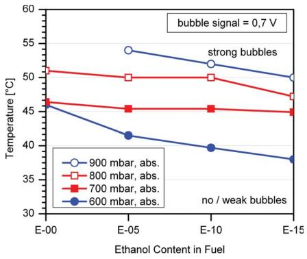
*Figure 52:* Temperature limits derived for the investigated ethanol abundancies and ambient pressure levels for the higher bubble intensity level of 0.7 V sensor readout.
