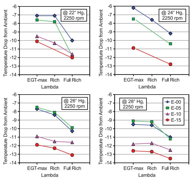
Figure 40: Temperature drop due to gasoline evaporation enthalpy in the intake manifold of the MORANE's Lycoming engine type O 360 A1A for various load conditions. The three states of air/fuel mixture settings can only be defined qualitatively and are likely to differ for the different admixture types due to slightly differing stoichiometric mass balances.
