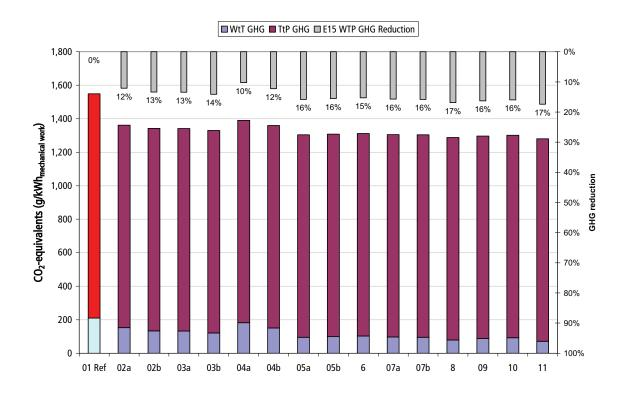
Figure 9: GHG emissions and emission reduction compared to reference WtP E15
