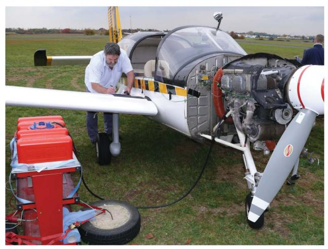
Figure 39: Morane icing test setup for operation with ethanol admixed fuels. The different gasoline compositions are taken from respective auxiliary tanks (red, left). They are fed by a bypass hose directly into the carburettor feed line. The aircraft is tied down to the ground with a strong rammed-in pole that is capable of supporting the full-power thrust of the engine.
