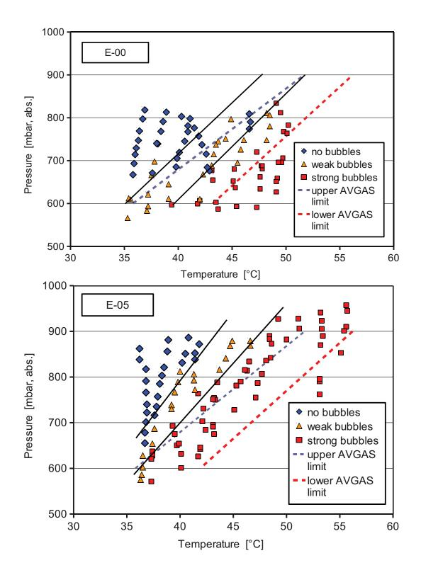
Figure 49: Bubble sensor readouts for a  $\{p,T\}$  scan of E-0 (top) and E-5 (bottom). Blue diamonds indicate a readout S < 0.3 V, orange triangles a value 0.3 V < S < 0.7 V, red squares indicate S > 0.7 V. Averaged region borders are sketched as black lines. Respective borders for AVGAS (cf. Fig. 48) are additionally shown as dashed lines.
