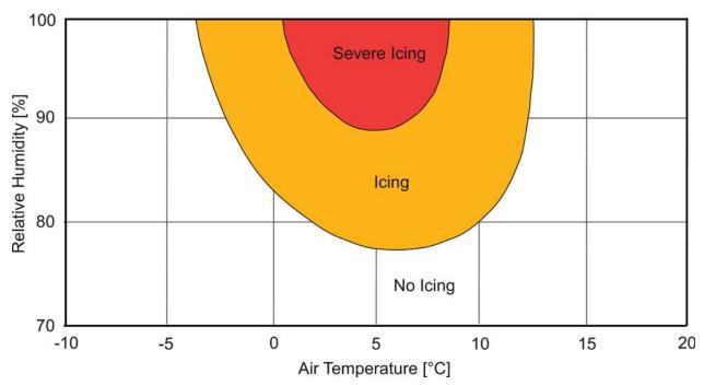
Figure 20: Temperature / humidity domains for increased danger of carburettor icing at ground atmospheric pressure, after [1]
