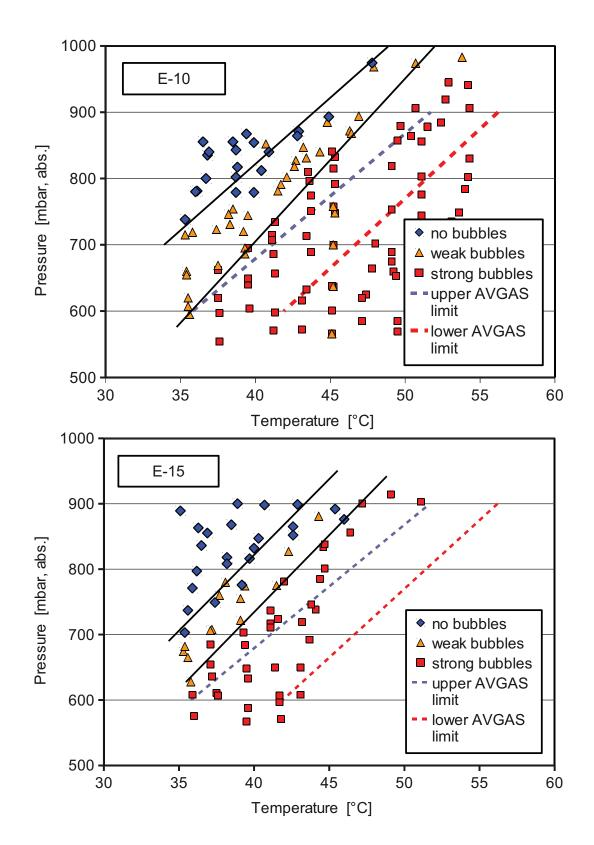
Figure 50: Bubble sensor readouts for a  $\{p,T\}$  scan of custom mixed E-10 (top) and E-15 (bottom). Blue diamonds indicate a readout S < 0.3 V, orange triangles a value 0.3 V < S < 0.7 V, red squares indicate S > 0.7 V. Averaged region borders are sketched as black lines. Respective borders for AVGAS (cf. Fig. 48) are additionally shown as dashed lines.
