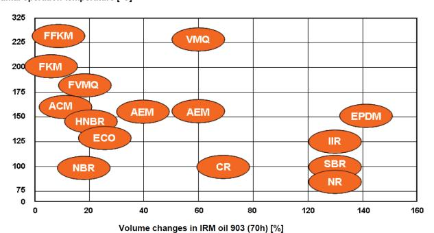
Figure 55: Oil resistance of elastomers
