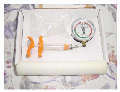
Figure 53: Hodges tester for gasoline volatility assessment.
