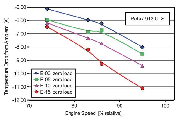
Figure 38: Temperature drop due to gasoline evaporation enthalpy in the intake manifold of the ROTAX 912 ULS engine under zero load conditions. Ambient conditions: 24.3°C, 98.4 kPa, 69.2 % rel. humidity
