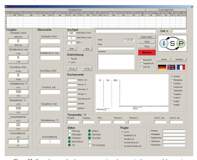
Figure 95: Example screen for the parameter setting of automatized test runs of the test rig
