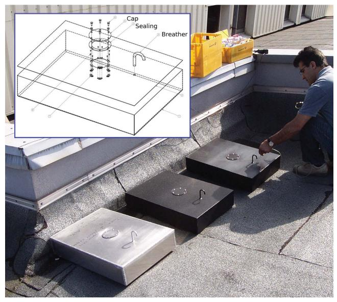
Figure 31: Custom made aircraft wing tank simulation vessels with comparative volume/surface ratio, used for long-term storaging experiments. Tanks were donated and stored by Gomolzig Flugzeug und Maschinenbau GmbH, Schwelm. Shown are the three exposed tanks stored on the roof.
