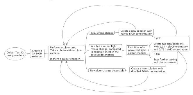
**Figure 69:** Sensitivity determination schema for an ethanol detection kit working on colour change reaction.
