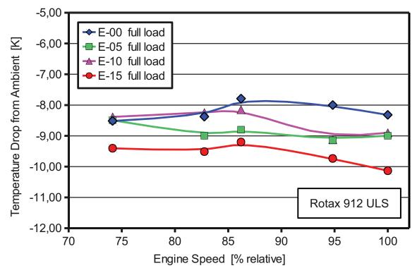
Figure 37: Temperature drop due to gasoline evaporation enthalpy in the intake manifold of the ROTAX 912 ULS engine under full load conditions. Ambient conditions: 24.3°C, 98.4 kPa, 69.2% rel. humidity
