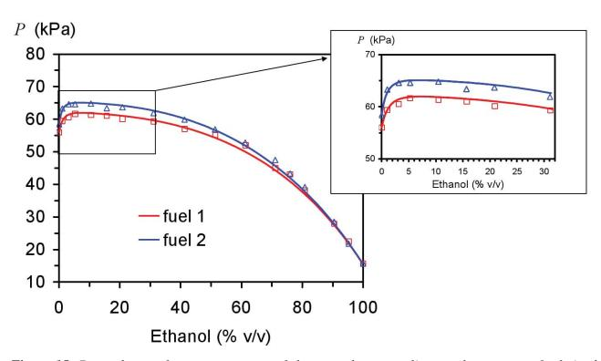
Figure 15: Dependence of vapour pressure of the same base gasoline on the amount of admixed EtOH, after [28].
