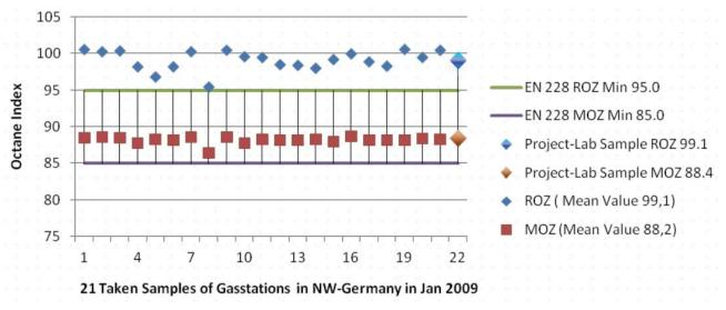
Figure 7: Octane numbers of 21 test samples taken at different gasoline stations in north-western Germany during January 2009. The 22<sup>nd</sup> entry shows the RON and MON values for the standard gasoline taken for all experiments conducted in the SIOBIA project (curtesy Total Deutschland GmbH)
