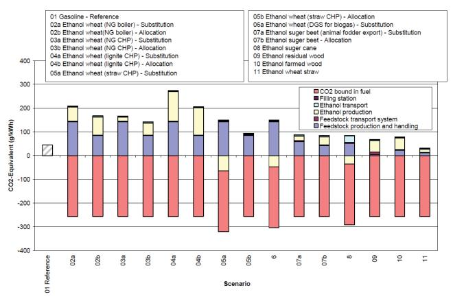
Figure 80: LBST well to tank greenhouse gas emission analysis results, comprising a variety of variants of process heat / steam generation for endothermic assisting processes (lignite cracking etc.). The various considered emissions  $(N_2O, CH_4)$  are introduced into the calculation as  $CO_2$  equivalents.
