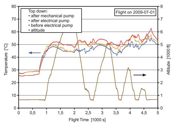
Figure 43: Development of fuel hose temperatures near to the enginge for a series of consecutive starts and fast touch-downs with AcUAS' MORANE. Deviating from the original flight card the zeniths were chosen consecutively lower.
