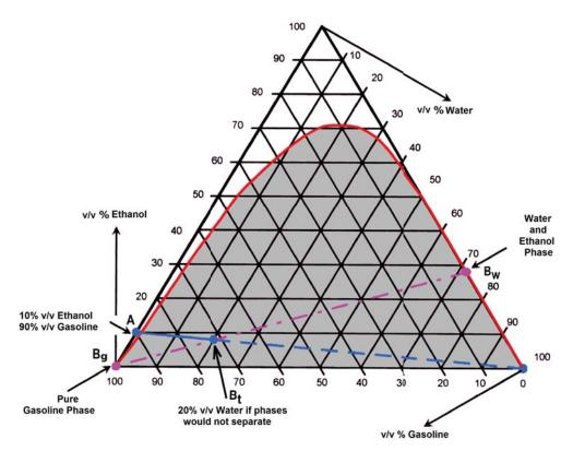
Figure 11: Ternary diagram for the substances gasoline, water and ethanol at 21 °C, after [31].
