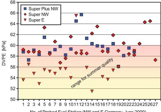
No. of Probed Fuel Station (NW and E Germany, June 2009)
