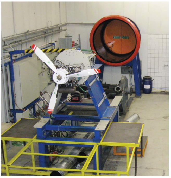
Figure 91: ROTAX 912 ULS on test rig
