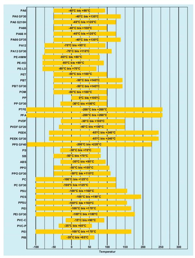
Figure 58: Temperature resistance of thermoplastics
