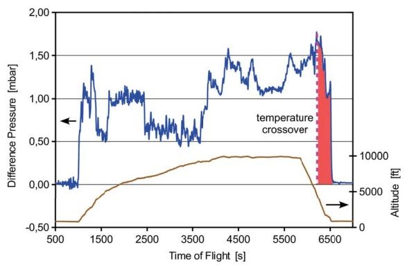
Figure 30: Air ingestion by tank ventilation, measured during a long-distance flight in one of MORANE's tank venting inlets. A positive value of the difference pressure indicates a flow into the tank. Humidity absorption endangered interval is painted red. For discussion see text.
