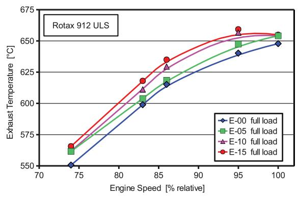
Figure 77: Rotax exhaust temperatures with ethanol admixed fuels. Unchanged carburettor settings for the different ethanol shares lead to slightly different actual fuel/air ratios in the comparation.
