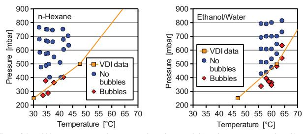
Figure 96: Bubble measurement observations for n-hexane (left) and an azeotropic ethanol/water mixture (right) in combination with the governing theoretical evaporation curve for the respective substance [17].
