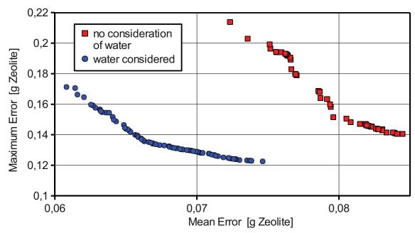
**Figure 75:** Zeolite water absorption evaluation. Shown are two pareto sets for the respective fit parameters with and without consideration of the influence of water. Both average error and maximum deviation from the measured data are well reduced if a water influence is taken into account.
