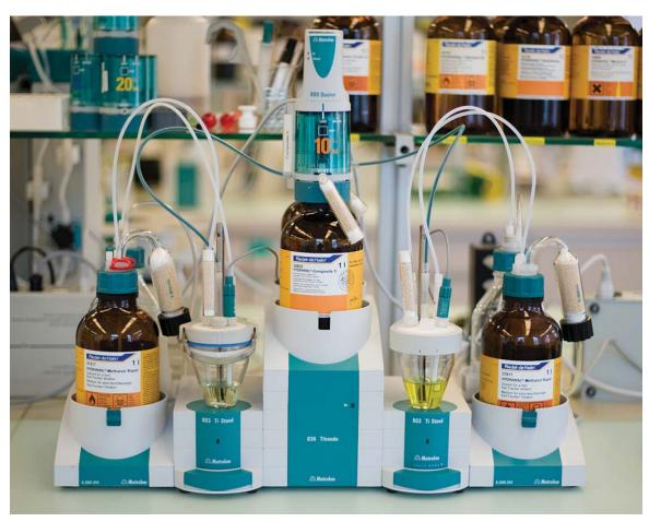
Figure 72: Setup for a water detection by a Karl-Fischer titration. (Image source: Wikipedia)
