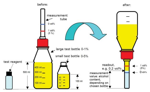
Figure 71: Maul's Fuel-Alk Tester (after http://www.daec.de/te/downfiles/Fuel-AlkTester.pdf).
