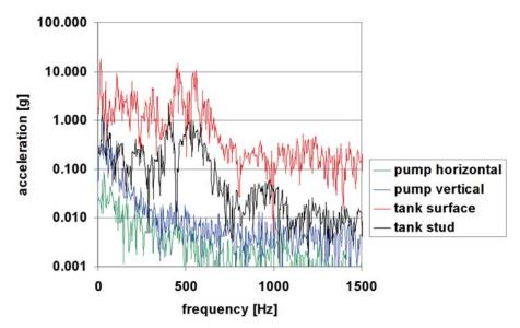
*Figure 45:* Vibration frequencies and strengths at various positions of the MORANE fuel system, take-off condition.
