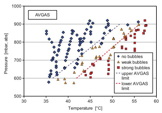
Figure 48: Bubble sensor readouts for a  $\{p,T\}$  scan of AVGAS. Blue diamonds indicate a readout S < 0.3 V, orange triangles a value 0.3 V < S < 0.7 V, red squares indicate S > 0.7 V.
