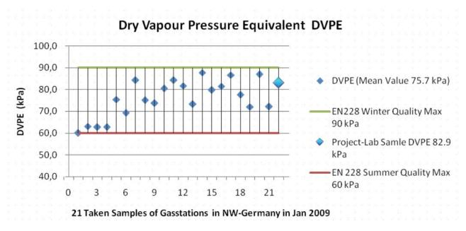
Figure 18: DVPE values of 21 test samples taken at different gasoline stations in north-western Germany during January 2009, curtesy Total Deutschland GmbH.
