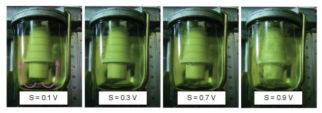
Figure 46: Collection of bubble strength images seen through the viewport, relating to respective sensor readout values. The arrows in the first image show the flow direction
