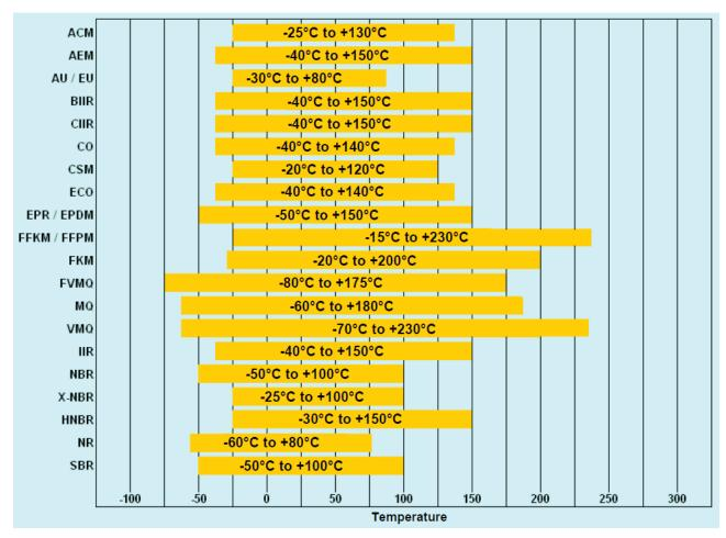
Figure 54: Temperature resistance of elastomers
