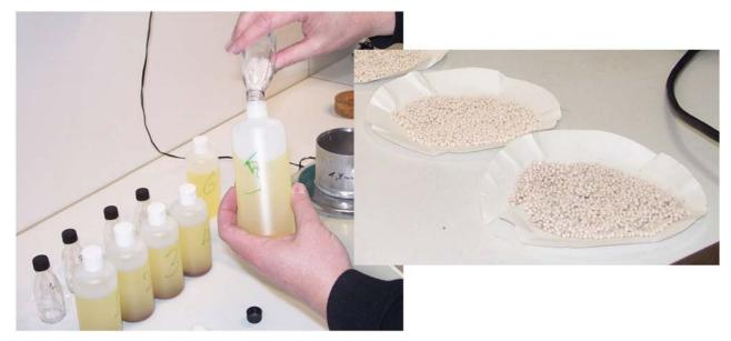
Figure 74: Zeolite water absorption experiment: Zeolite granules are given to gasoline probes (left). After vigorous shaking the zeolite is filtered, and the filter residues are weighed after some time of gasoline evaporative drying. Image right shows slightly differently coloured filtering samples with differing dry times.
