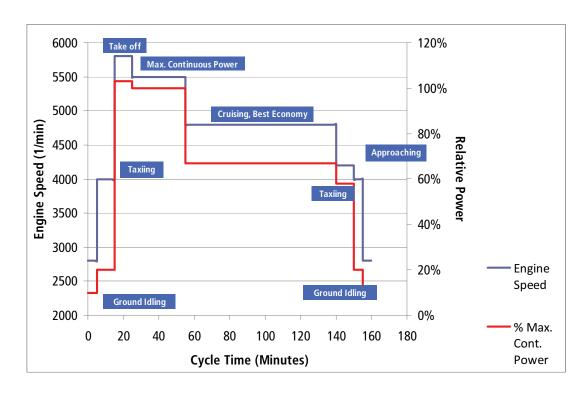
Figure 5: LTO cycle for engine emission measurements
