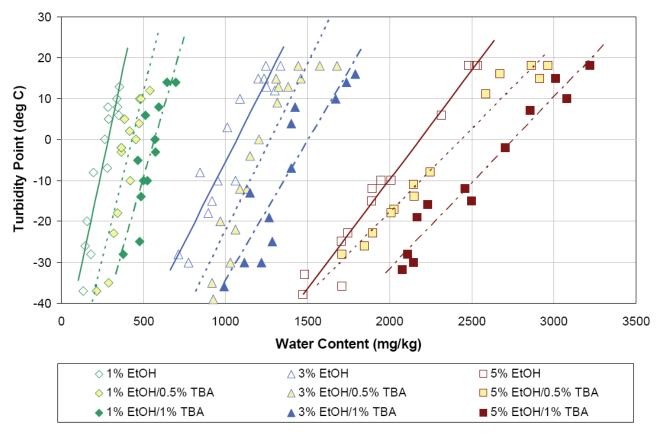
Figure 12: Maximum water concentrations in different gasoline/ethanol mixtures as a function of temperature, after [28]. By cool-down experiments the onset of turbidity was measured as a function of fuel composition, denominating the limit of water acceptance. Percentages are given as m/m values. Explanation see text.
