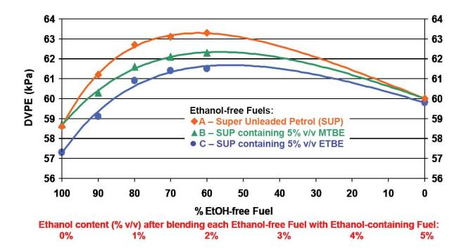
Each Ethanol-free Fuel was blended with an Ethanol-containing Fuel (5% v/v ethanol & 1250ppm water) before the DVPE of the final blend was measured
