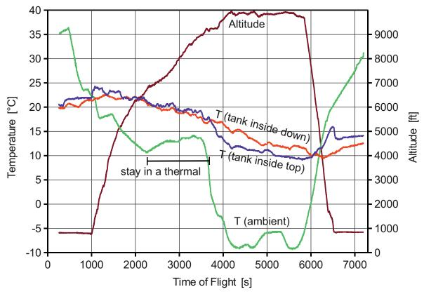
Figure 28: Temperature developments at different positions inside the fuel tank of the MORANE
