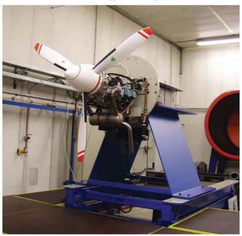
Figure 4: Piston engine test stand at FH Aachen
