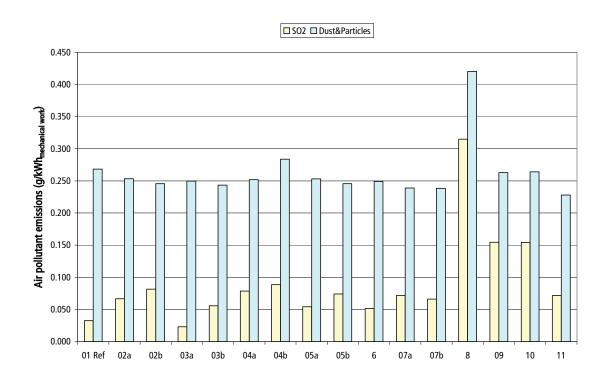
Figure 17: SO<sub>2</sub> and dust/PM WtT emissions for E15
